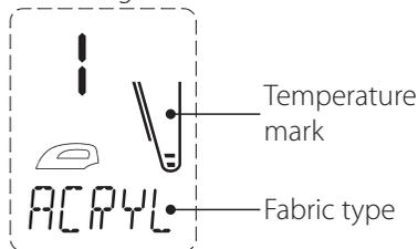
4. When your set temperature is reached, the iron will beep once and the fabric type will stop flashing.
